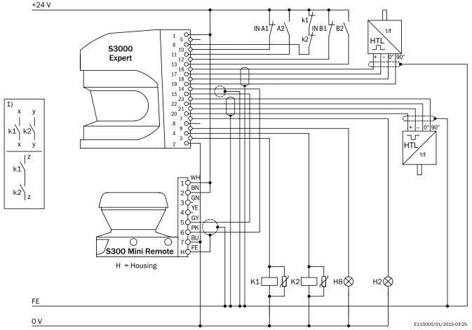
S3000 Expert with S300 Mini Remote in an EFI system with relays/contactors Operating mode: without restart interlock with external device monitoring
