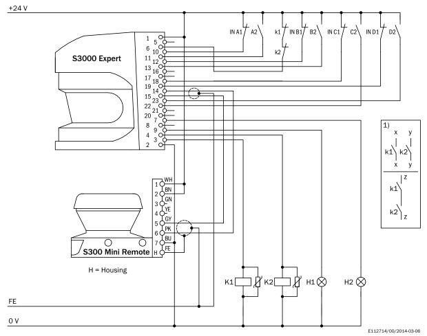
${\tt S3000\ Expert\ with\ S300\ Mini\ Remote\ in\ an\ EFI\ system\ with\ relays/contactors}$
