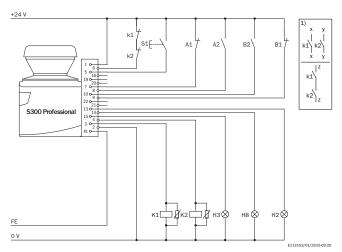
S300 Professional in connection with relays/contactors
