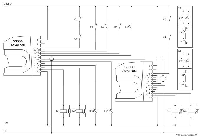
S3000 Advanced with S3000 Advanced in conjunction with relays/contactors
