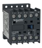
TeSys K contactor - 3P - AC-3 <= 440 V 9 A - 1 NO aux. - 400...415 V AC coil
