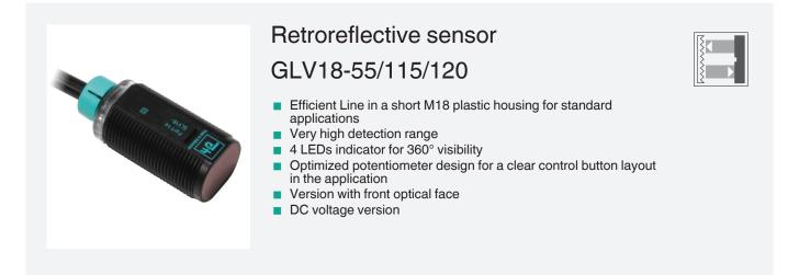
Retroreflective sensor with polarization filter, M18 threaded housing design, plastic housing, front optical face, 4 m detection range, red light, light/dark on, DC version, 2 PNP outputs, fixed cable
