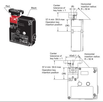
\* Insertion radii apply when the rotational center of the Operation Key is in line with a line extending from the front or top Head surface.
