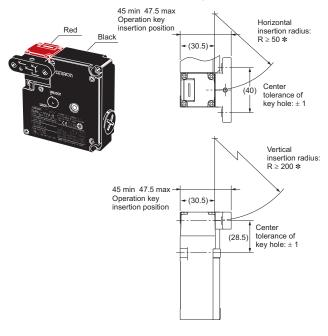
D4NL + D4DS-K3 (with Top-inserted Operation Key)
