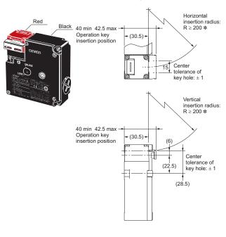
D4NL + D4DS-K2 (with Top-inserted Operation Key)
