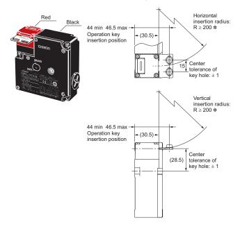
D4NL + D4DS-K1 (with Top-inserted Operation Key)
