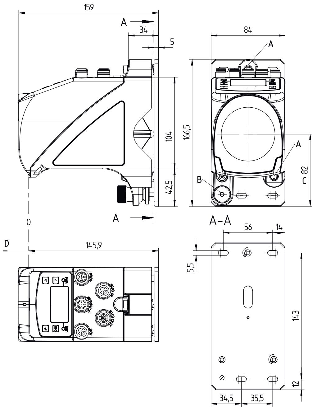
A M5 screw for alignment
