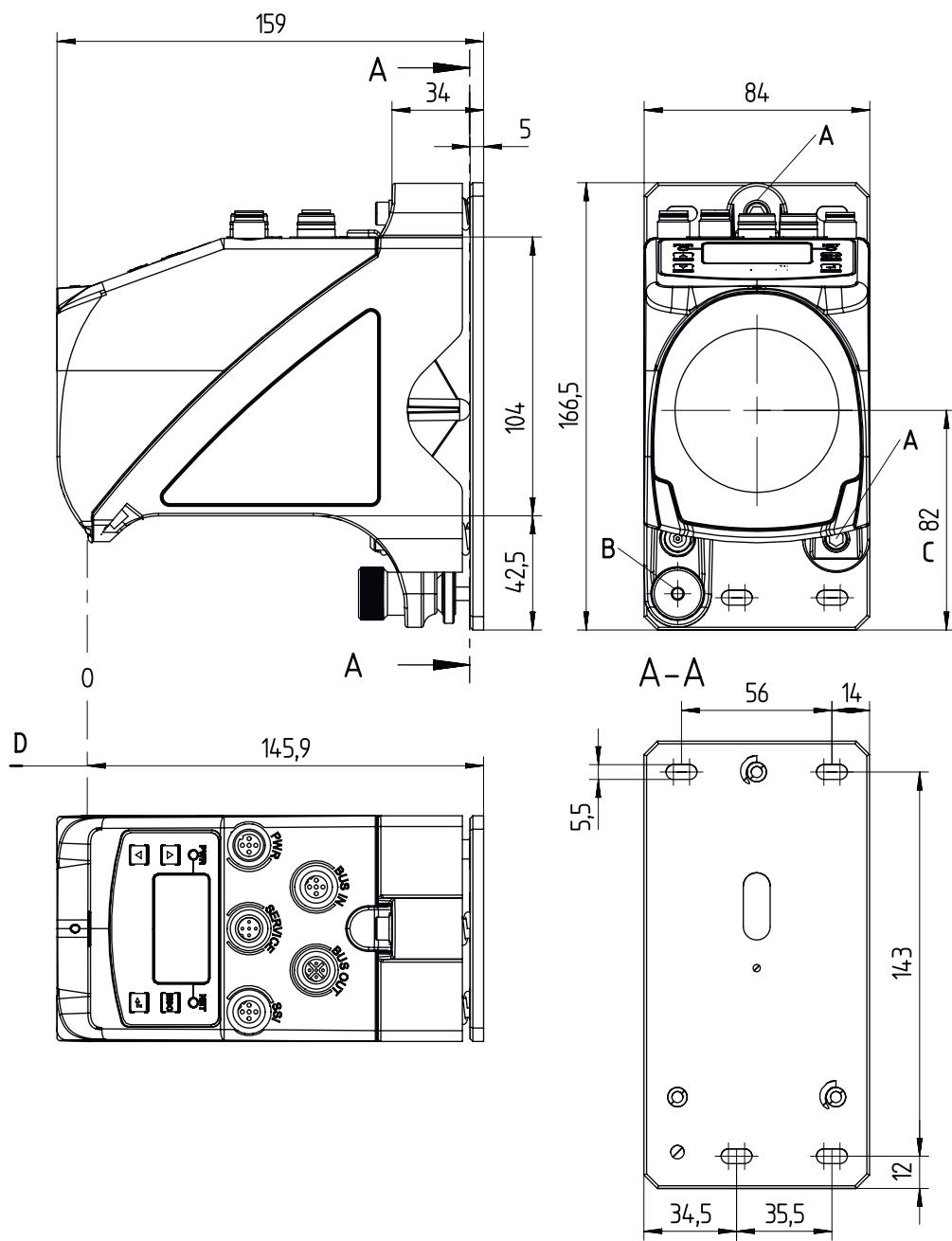
A M5 screw for alignment
