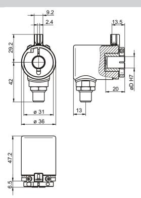
With flange connector M12 and torque pin
